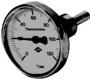
Fig. 20 Dial Diameter : 100 mm. Case : steel Galvanised Wetted Part : Brass Bulb : Brass/Steel Accuracy : +/- 4% Bulb length : 100 mm. Connection : 1/2" BSP Position : Back Range : 0-120°C, 0-400°C
